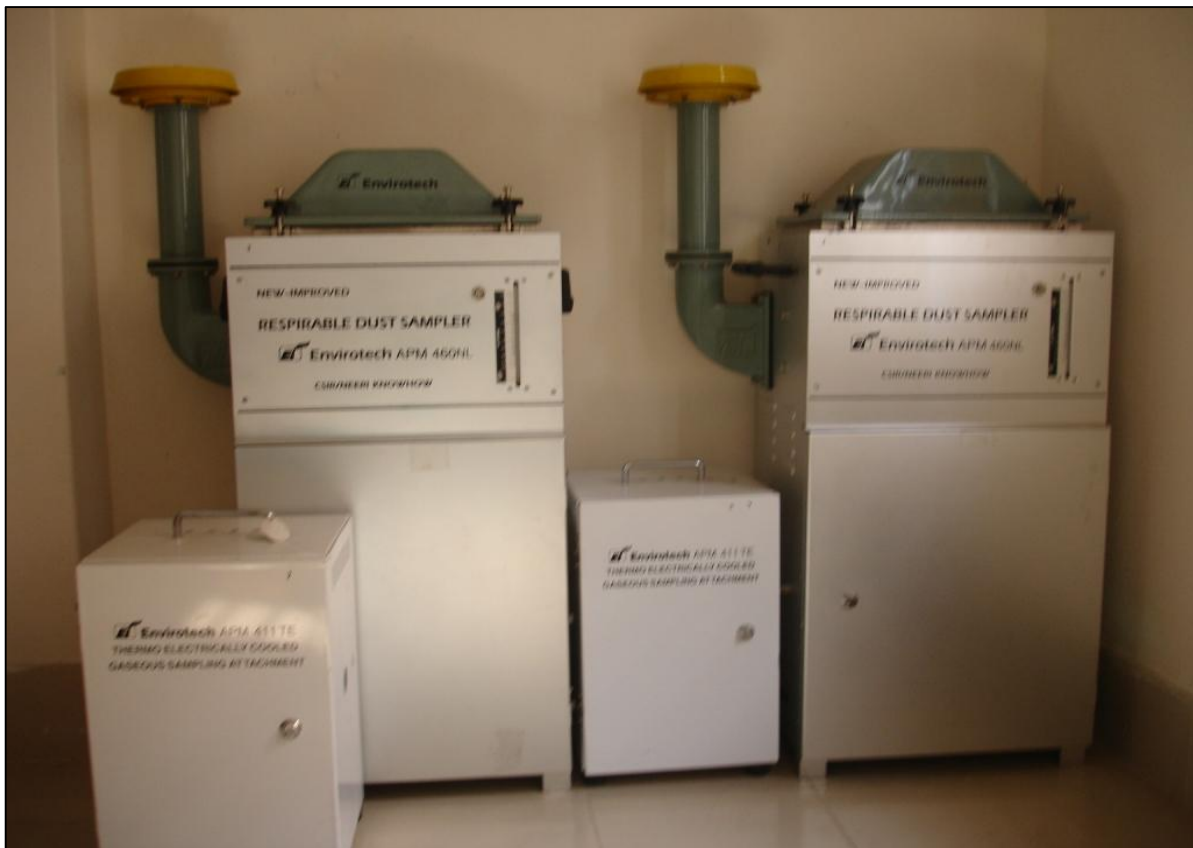
Photo-4.1: Respirable Dust Sampler for SPM, PM 10 , SO 2 , NOx measurement
