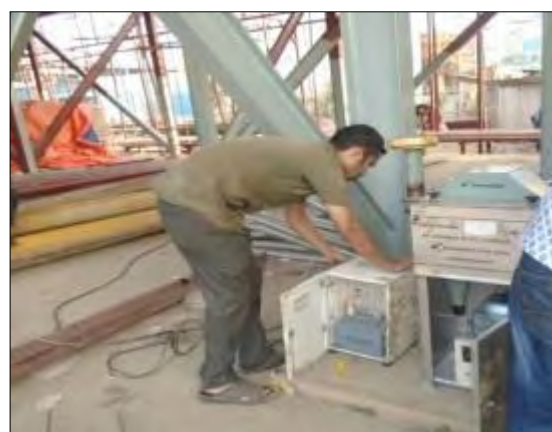
Photo 4.1: Respirable Dust Sampler for SPM, PM 10 and SO 2 , NO x , CO measurement instruments and measurement activities.
