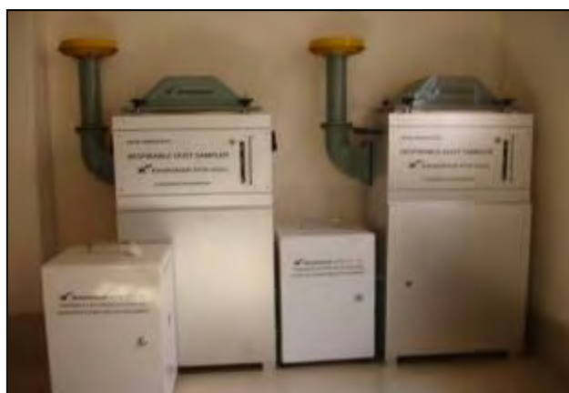
Photo 4.1: Respirable Dust Sampler for SPM, PM 10 and SO 2 , NO x , CO measurement instruments and measurement activities.
