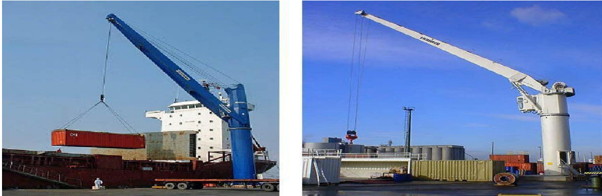
Figure 3.12: Fixed Cargo Cranes (FCCs) will be fitted on fixed pedestals on the quaysides
