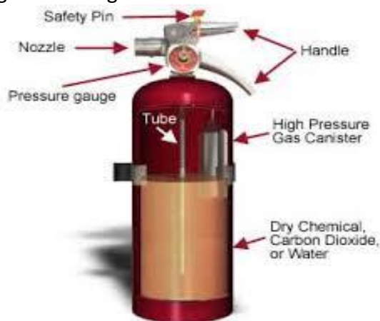
Figure 8.1: Different parts of portable extinguisher
