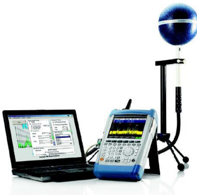
Figure 4.12: Robi's EMF radiation measuring instrument
