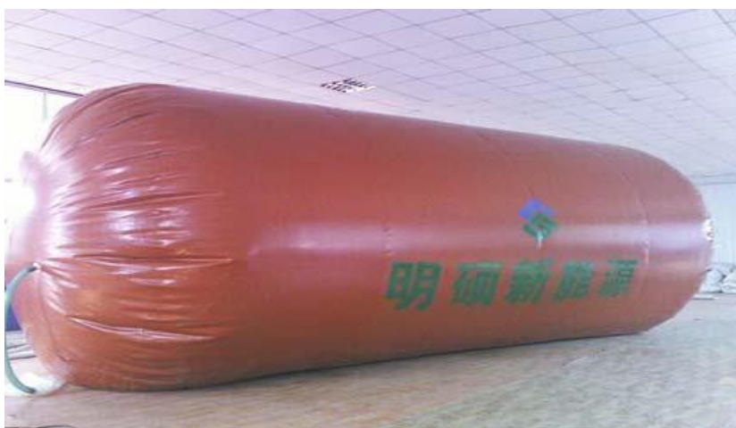
Figure 3.8: Red Mud Biogas Storage Bag
